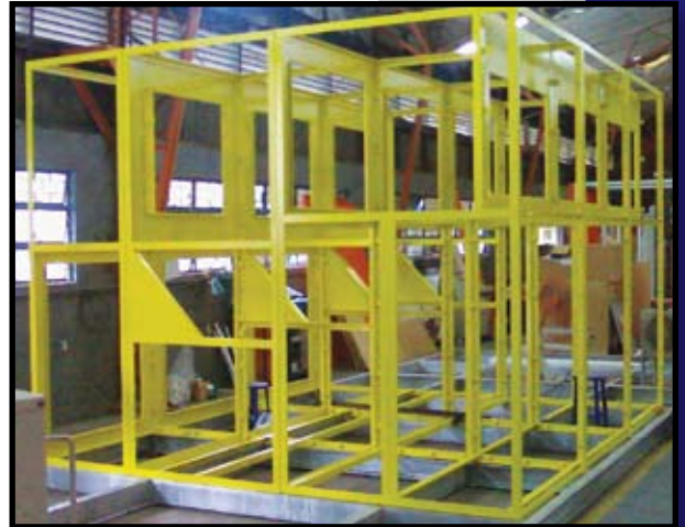
36 kV MVSG Structural Assembly
